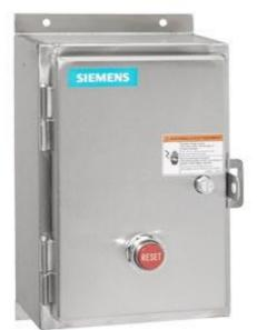
Non-reversing motor starter Size 3 Three phase full voltage Amb compensate bimetal OLrelay Contactor amp rating 90 AMP Non-combination type Encl NEMA type 4X 304 S-steel Water/dust tight non-corrosive Extra-wide enclosure
