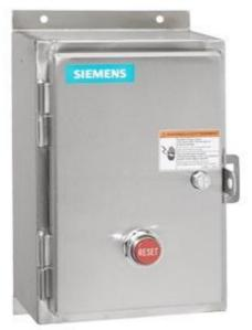
Non-reversing motor starter Size 3 Three phase full voltage Amb compensate bimetal OLrelay Contactor amp rating 90 AMP 208VAC 60HZ coil Non-combination type Encl NEMA type 4X 304 S-steel Water/dust tight non-corrosive Extra-wide enclosure
