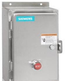
Non-reversing motor starter Size 3 Three phase full voltage Amb compensate bimetal OLrelay Contactor amp rating 90 AMP 240VAC 50HZ / 277VAC 60HZ coil Non-combination type Encl NEMA type 4X 304 S-steel Water/dust tight non-corrosive Extra-wide enclosure
