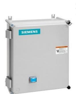
Non-reversing motor starter Size 3 Three phase full voltage Solidstate overload relay OLRelay amp range 25-100A Non-combination type Encl NEMA type 4X Fiberglass Water/dust tight non-corrosive Standard width enclosure
