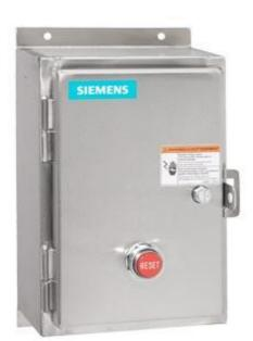
Non-reversing motor starter Size 4 Three phase full voltage Solidstate overload relay OLRelay amp range 50-200A Non-combination type Encl NEMA type 4X 316 S-steel Water/dust tight non-corrosive Standard width enclosure
