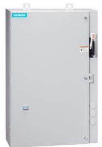
Non-reversing motor starter Size 0 Three phase full voltage Amb compensate bimetal OLrelay Contactor amp rating 18Amp Combination type 30Amp fusible disconnect 30 Amp /600V fuse clip Enclosure NEMA type 4/12 Water/dust tight weather proof Extra-wide enclosure
