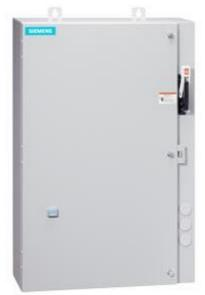
Non-reversing motor starter Size 0 Three phase full voltage Amb compensate bimetal OLrelay Contactor amp rating 18Amp 110-120/220-240VAC 60HZ coil Combination type 30Amp non-fusible disconnect Enclosure NEMA type 4/12 Water/dust tight weather proof Extra-wide enclosure
