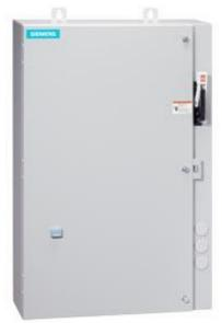
Non-reversing motor starter Size 0 Three phase full voltage Amb compensate bimetal OLrelay Contactor amp rating 18Amp 220-240/440-480VAC 60HZ coil Combination type 30Amp fusible disconnect 30 Amp /600V fuse clip Enclosure NEMA type 4/12 Water/dust tight weather proof Extra-wide enclosure
