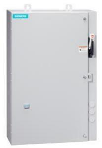
Non-reversing motor starter Size 0 Three phase full voltage Amb compensate bimetal OLrelay Contactor amp rating 18Amp 220-240/440-480VAC 60HZ coil Combination type 30Amp non-fusible disconnect Enclosure NEMA type 4/12 Water/dust tight weather proof Extra-wide enclosure
