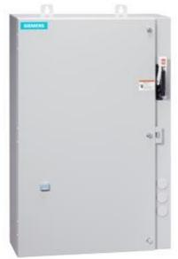
Non-reversing motor starter Size 0 Three phase full voltage Amb compensate bimetal OLrelay Contactor amp rating 18Amp 208VAC 60HZ coil Combination type 30Amp fusible disconnect 30 Amp /600V fuse clip Enclosure NEMA type 4/12 Water/dust tight weather proof Extra-wide enclosure
