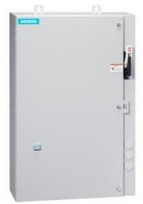
Non-reversing motor starter, Size 0, Three phase full voltage, Amb compensate bimetal OLrelay Contactor amp rating 18Amp 110V 50HZ / 120V 60HZ coil, Combination type, 30Amp fusible disconnect 30 Amp /600V fuse clip, Enclosure NEMA type 4/12, Water/dust tight for outdoors, Extra-wide enclosure
