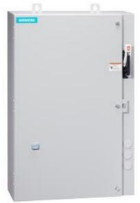
Non-reversing motor starter Size 0 Three phase full voltage Amb compensate bimetal OLrelay Contactor amp rating 18Amp 110VAC 50HZ / 120VAC 60HZ coil Combination type 30Amp non-fusible disconnect Enclosure NEMA type 4/12 Water/dust tight weather proof Extra-wide enclosure
