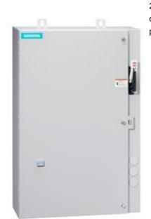
Non-reversing motor starter Size 0 Three phase full voltage Amb compensate bimetal OLrelay Contactor amp rating 18Amp 190-220/220-240V 50/60HZ coil Combination type 30Amp non-fusible disconnect Enclosure NEMA type 4/12 Water/dust tight weather proof Extra-wide enclosure
