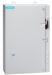
Non-reversing motor starter Size 0 Three phase full voltage Amb compensate bimetal OLrelay Contactor amp rating 18Amp Combination type 30Amp fusible disconnect 30Amp / 250V fuse clip Enclosure NEMA type 4/12 Water/dust tight weather proof Extra-wide enclosure
