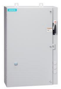
Non-reversing motor starter Size 0 Three phase full voltage Amb compensate bimetal OLrelay Contactor amp rating 18Amp 380-440/440-480V 50/60HZ coil Combination type 30Amp non-fusible disconnect Enclosure NEMA type 4/12 Water/dust tight weather proof Extra-wide enclosure
