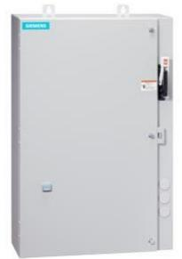
Non-reversing motor starter Size 0 Three phase full voltage Amb compensate bimetal OLrelay Contactor amp rating 18Amp 24VAC 50-60HZ coil Combination type 30Amp fusible disconnect 30 Amp /600V fuse clip Enclosure NEMA type 4/12 Water/dust tight weather proof Extra-wide enclosure
