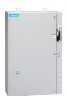
Non-reversing motor starter Size 0 Three phase full voltage Amb compensate bimetal OLrelay Contactor amp rating 18Amp 240VAC 50HZ / 277VAC 60HZ coil Combination type 30Amp non-fusible disconnect Enclosure NEMA type 4/12 Water/dust tight weather proof Extra-wide enclosure
