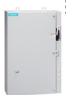
Non-reversing motor starter Size 0 Three phase full voltage Amb compensate bimetal OLrelay Contactor amp rating 18Amp 24Vdc coil Combination type 30Amp fusible disconnect 30Amp / 250V fuse clip Enclosure NEMA type 4/12 Water/dust tight weather proof Extra-wide enclosure
