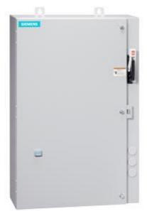
Non-reversing motor starter Size 0 Three phase full voltage Amb compensate bimetal OLrelay Contactor amp rating 18Amp 24Vdc coil Combination type 30Amp non-fusible disconnect Enclosure NEMA type 4/12 Water/dust tight weather proof Extra-wide enclosure
