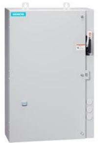
Non-reversing motor starter Size 0 Three phase full voltage Amb compensate bimetal OLrelay Contactor amp rating 18Amp 110-120/220-240VAC 60HZ coil Combination type 30Amp fusible disconnect 30Amp / 250V fuse clip Encl NEMA type 4X 304 S-steel Water/dust tight non-corrosive Extra-wide enclosure
