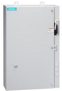
Non-reversing motor starter Size 0 Three phase full voltage Amb compensate bimetal OLrelay Contactor amp rating 18Amp Combination type 30Amp fusible disconnect 30Amp / 250V fuse clip Encl NEMA type 4X 304 S-steel Water/dust tight non-corrosive Extrawide enclosure
