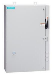
Non-reversing motor starter Size 0 Three phase full voltage Amb compensate bimetal OLrelay Contactor amp rating 18Amp Combination type 30Amp non-fusible disconnect Encl NEMA type 4X 304 S-steel Water/dust tight non-corrosive Extra-wide enclosure
