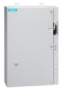
Non-reversing motor starter Size 0 Three phase full voltage Amb compensate bimetal OLrelay Contactor amp rating 18Amp 220-240/440-480VAC 60HZ coil Combination type 30Amp fusible disconnect 30 Amp /600V fuse clip Encl NEMA type 4X 304 S-steel Water/dust tight non-corrosive Extra-wide enclosure
