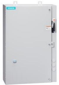
Non-reversing motor starter Size 0 Three phase full voltage Amb compensate bimetal OLrelay Contactor amp rating 18Amp 220-240/440-480VAC 60HZ coil Combination type 30Amp non-fusible disconnect Encl NEMA type 4X 304 S-steel Water/dust tight non-corrosive Extra-wide enclosure
