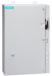
Non-reversing motor starter Size 0 Three phase full voltage Amb compensate bimetal OLrelay Contactor amp rating 18Amp 208VAC 60HZ coil Combination type 30Amp fusible disconnect 30 Amp /600V fuse clip Encl NEMA type 4X 304 S-steel Water/dust tight non-corrosive Extra-wide enclosure
