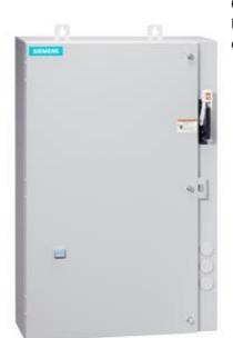
Non-reversing motor starter Size 0 Three phase full voltage Amb compensate bimetal OLrelay Contactor amp rating 18Amp 208VAC 60HZ coil Combination type 30Amp non-fusible disconnect Encl NEMA type 4X 304 S-steel Water/dust tight non-corrosive Extra-wide enclosure
