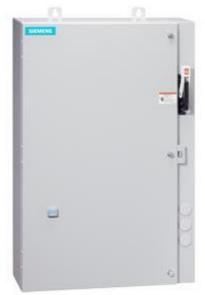
Non-reversing motor starter Size 0 Three phase full voltage Amb compensate bimetal OLrelay Contactor amp rating 18Amp 550/575-600 50/60HZ coil Combination type 30Amp fusible disconnect 30Amp / 250V fuse clip Encl NEMA type 4X 304 S-steel Water/dust tight non-corrosive Extra-wide enclosure
