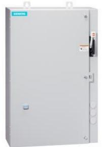
Non-reversing motor starter Size 0 Three phase full voltage Amb compensate bimetal OLrelay Contactor amp rating 18Amp 550/575-600 50/60HZ coil Combination type 30Amp non-fusible disconnect Encl NEMA type 4X 304 S-steel Water/dust tight non-corrosive Extrawide enclosure
