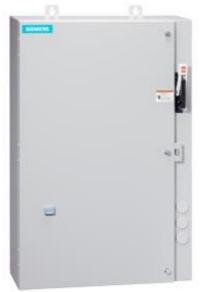
Non-reversing motor starter Size 0 Three phase full voltage Amb compensate bimetal OLrelay Contactor amp rating 18Amp 110VAC 50HZ / 120VAC 60HZ coil Combination type 30Amp non-fusible disconnect Encl NEMA type 4X 304 S-steel Water/dust tight non-corrosive Extra-wide enclosure
