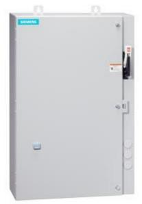
Non-reversing motor starter Size 0 Three phase full voltage Amb compensate bimetal OLrelay Contactor amp rating 18Amp 190-220/220-240V 50/60HZ coil Combination type 30Amp fusible disconnect 30Amp / 250V fuse clip Encl NEMA type 4X 304 S-steel Water/dust tight non-corrosive Extra-wide enclosure
