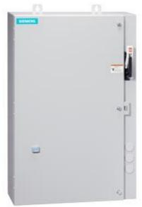
Non-reversing motor starter Size 0 Three phase full voltage Amb compensate bimetal OLrelay Contactor amp rating 18Amp 380-440/440-480V 50/60HZ coil Combination type 30Amp non-fusible disconnect Encl NEMA type 4X 304 S-steel Water/dust tight non-corrosive Extra-wide enclosure
