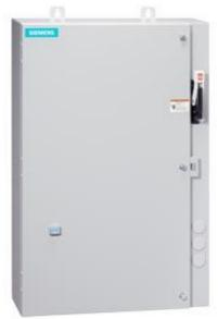
Non-reversing motor starter Size 0 Three phase full voltage Amb compensate bimetal OLrelay Contactor amp rating 18Amp 24VAC 50-60HZ coil Combination type 30Amp fusible disconnect 30Amp / 250V fuse clip Encl NEMA type 4X 304 S-steel Water/dust tight non-corrosive Extra-wide enclosure
