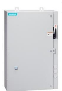
Non-reversing motor starter Size 0 Three phase full voltage Amb compensate bimetal OLrelay Contactor amp rating 18Amp 24VAC 50-60HZ coil Combination type 30Amp fusible disconnect 30 Amp /600V fuse clip Encl NEMA type 4X 304 S-steel Water/dust tight noncorrosive Extra-wide enclosure
