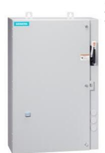
Non-reversing motor starter Size 0 Three phase full voltage Amb compensate bimetal OLrelay Contactor amp rating 18Amp 240VAC 50HZ / 277VAC 60HZ coil Combination type 30Amp non-fusible disconnect Encl NEMA type 4X 304 S-steel Water/dust tight non-corrosive Extra-wide enclosure
