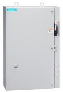
Non-reversing motor starter Size 0 Three phase full voltage Amb compensate bimetal OLrelay Contactor amp rating 18Amp 24Vdc coil Combination type 30Amp fusible disconnect 30Amp / 250V fuse clip Encl NEMA type 4X 304 S-steel Water/dust tight non-corrosive Extrawide enclosure
