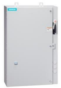
Non-reversing motor starter Size 0 Three phase full voltage Amb compensate bimetal OLrelay Contactor amp rating 18Amp 24Vdc coil Combination type 30Amp fusible disconnect 30Amp / 250V fuse clip Encl NEMA type 4X 304 S-steel Water/dust tight non-corrosive Extrawide enclosure
