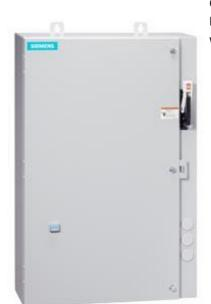
Non-reversing motor starter Size 0 Three phase full voltage Amb compensate bimetal OLrelay Contactor amp rating 18Amp 24Vdc coil Combination type 30Amp fusible disconnect 30 Amp /600V fuse clip Encl NEMA type 4X 304 S-steel Water/dust tight non-corrosive Extrawide enclosure
