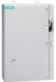
Non-reversing motor starter Size 0 Three phase full voltage Amb compensate bimetal OLrelay Contactor amp rating 18Amp 24Vdc coil Combination type 30Amp fusible disconnect 30 Amp /600V fuse clip Encl NEMA type 4X 304 S-steel Water/dust tight non-corrosive Extrawide enclosure
