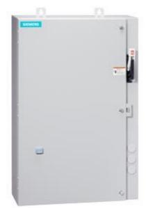
Non-reversing motor starter Size 0 Three phase full voltage Amb compensate bimetal OLrelay Contactor amp rating 18Amp 24Vdc coil Combination type 30Amp non-fusible disconnect Encl NEMA type 4X 304 S-steel Water/dust tight non-corrosive Extra-wide enclosure
