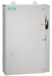
Non-reversing motor starter Size 0 Three phase full voltage Amb compensate bimetal OLrelay Contactor amp rating 18Amp Combination type 30Amp fusible disconnect 30Amp / 250V fuse clip Encl NEMA type 4X 316 S-steel Water/dust tight non-corrosive Extrawide enclosure
