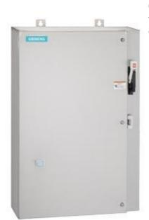
Non-reversing motor starter Size 0 Three phase full voltage Amb compensate bimetal OLrelay Contactor amp rating 18Amp 208VAC 60HZ coil Combination type 30Amp fusible disconnect 30Amp / 250V fuse clip Encl NEMA type 4X 316 S-steel Water/dust tight noncorrosive Extra-wide enclosure
