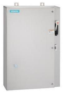
Non-reversing motor starter Size 0 Three phase full voltage Amb compensate bimetal OLrelay Contactor amp rating 18Amp 208VAC 60HZ coil Combination type 30Amp fusible disconnect 30 Amp /600V fuse clip Encl NEMA type 4X 316 S-steel Water/dust tight non-corrosive Extra-wide enclosure
