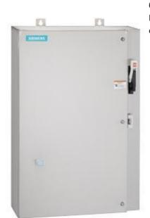
Non-reversing motor starter Size 0 Three phase full voltage Amb compensate bimetal OLrelay Contactor amp rating 18Amp 208VAC 60HZ coil Combination type 30Amp non-fusible disconnect Encl NEMA type 4X 316 S-steel Water/dust tight non-corrosive Extra-wide enclosure
