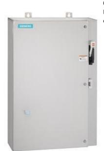
Non-reversing motor starter Size 0 Three phase full voltage Amb compensate bimetal OLrelay Contactor amp rating 18Amp 208VAC 60HZ coil Combination type 30Amp non-fusible disconnect Encl NEMA type 4X 316 S-steel Water/dust tight non-corrosive Extra-wide enclosure
