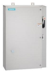
Non-reversing motor starter Size 0 Three phase full voltage Amb compensate bimetal OLrelay Contactor amp rating 18Amp 110VAC 50HZ / 120VAC 60HZ coil Combination type 30Amp fusible disconnect 30Amp / 250V fuse clip Encl NEMA type 4X 316 S-steel Water/dust tight non-corrosive Extra-wide enclosure
