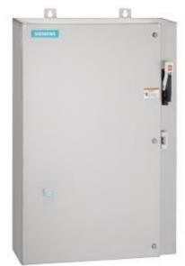
Non-reversing motor starter Size 0 Three phase full voltage Amb compensate bimetal OLrelay Contactor amp rating 18Amp Combination type 30Amp non-fusible disconnect Encl NEMA type 4X 316 S-steel Water/dust tight non-corrosive Extra-wide enclosure
