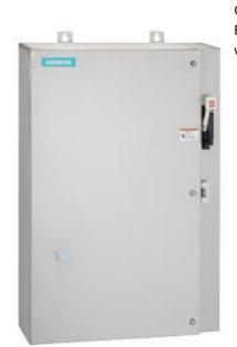
Non-reversing motor starter Size 0 Three phase full voltage Amb compensate bimetal OLrelay Contactor amp rating 18Amp Combination type 30Amp fusible disconnect 30 Amp /600V fuse clip Encl NEMA type 4X 316 S-steel Water/dust tight non-corrosive Extrawide enclosure
