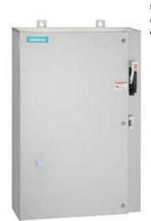
Non-reversing motor starter Size 0 Three phase full voltage Amb compensate bimetal OLrelay Contactor amp rating 18Amp 24VAC 50-60HZ coil Combination type 30Amp fusible disconnect 30 Amp /600V fuse clip Encl NEMA type 4X 316 S-steel Water/dust tight noncorrosive Extra-wide enclosure
