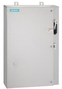
Non-reversing motor starter Size 0 Three phase full voltage Amb compensate bimetal OLrelay Contactor amp rating 18Amp 24VAC 50-60HZ coil Combination type 30Amp non-fusible disconnect Encl NEMA type 4X 316 S-steel Water/dust tight non-corrosive Extra-wide enclosure
