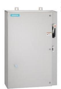
Non-reversing motor starter Size 0 Three phase full voltage Amb compensate bimetal OLrelay Contactor amp rating 18Amp 240VAC 50HZ / 277VAC 60HZ coil Combination type 30Amp fusible disconnect 30Amp / 250V fuse clip Encl NEMA type 4X 316 S-steel Water/dust tight non-corrosive Extra-wide enclosure
